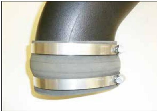
14. Slide the provided hump coupler completely onto the intake tube with the hose clamps as shown.
